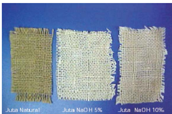
Fig. 7 Jute fibres after alkali treatment.
